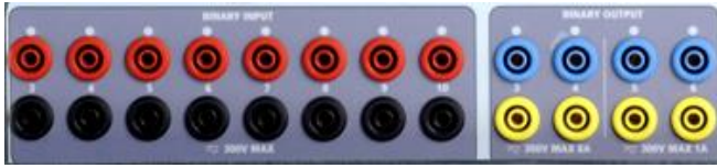
Figure 103 “P” Option Binary Inputs 3 to 10 and Binary Outputs 3 to 6
